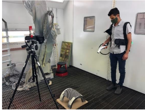
Figure 3: A sample is stretched over a curved surface on the ground, and sprayed at 45°
