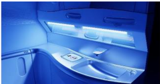
Figure 6: Boeing product development concept of Far-UV 222 nm implementation in a 787 lavatory
